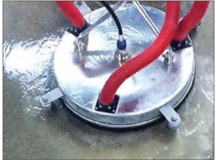
This allows the OBS-D to reach hydrocarbons deep within the concrete, bind with them, and “float” them to the surface for removal. Most floor spinners have vacuum attachments so that wastewater can be vacuumed up and contained for disposal in accordance with federal, state and local hazardous material regulations. This cleaning process may need to be repeated several times, depending on the level of contamination.
