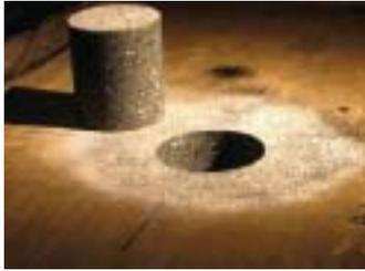
In order to properly determine the level, depth and type of contamination, core testing must be conducted. AC Tech recommends that short cores (2" deep x 3" dia.) be taken and sent to an independent lab for analysis via Infra-Red Spectroscopy, Ion Chromatography and X-Ray Diffraction. This data will help our technical staff produce precise recommendations.
