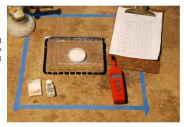
If quantitative assessment indicates moisture vapor emissions, building trades experienced decades of qualitative difficulties with the Calcium Chloride moisture test. In fact, moisture-plagued concrete slabs certified by ASTM F1869 protocol proved to be a patterned and persistent challenge to the concrete flooring industry – so much so that industry professionals began to investigate the scientific integrity of the Calcium Chloride moisture test and came up with the following three problems:
