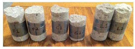
Bag each core as soon as it is taken to avoid any accidental contamination from outside sources. Pack in appropriate shipping container to avoid breakage during transit to the selected lab.
