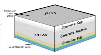
In cases where the concrete has been water cured or exposed to weathering for several weeks, and sometimes years, a carbonation layer forms on the cap and the surface pH may
