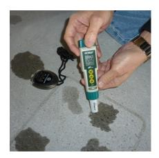
Using pH test papers (left) and an electronic pH tester (right) to determine pH of surface. Concrete surface must be free of all coatings, coverings, adhesive, carbonation layer etc. to get an accurate reading. ASTM F710 covers pH testing in concrete.
